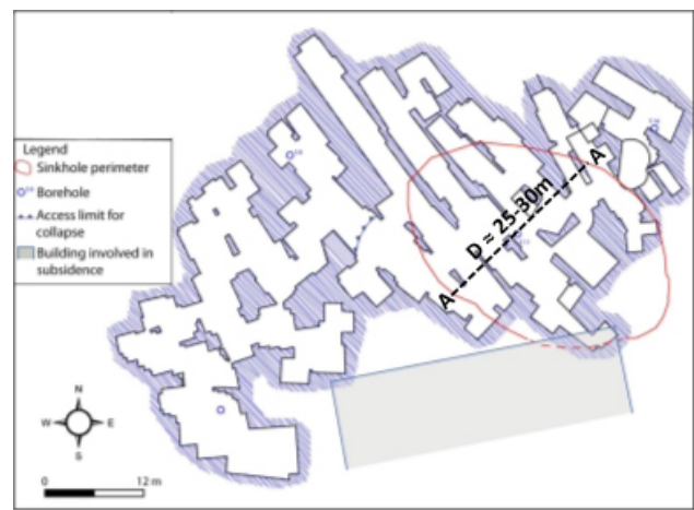
Figure 9. Plan of the Marsala underground quarry, with indication of the sinkhole area (adapted from Vattano et al., 2013).
